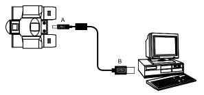
Fig. 2: Connecting the USB cable.
